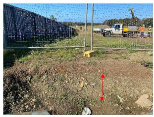
Looking east at excavated profile on boundary of Lot 208 and 400 exposing topsoil overlaying site won gravel fill to 0.7m.
